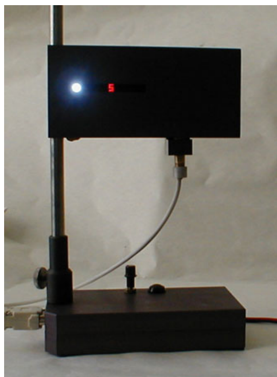
Figure 3C. Photograph of working prototype of the Halometer DG tester. The instrument can be used in the pre-testing examination room of optometrist and ophthalmologists offices and also for self testing.
